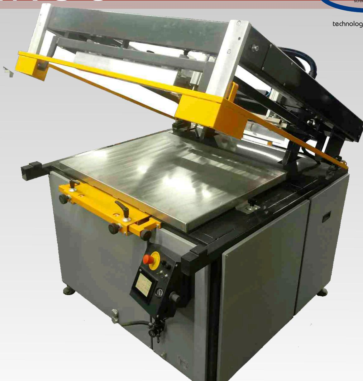
FARGO is flatbed machine with angle lifted print head. Screen lifting and carriage drive made with moto-reducer driven by frequency converter.
